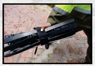
You can hold and deploy the Strip various ways by holding onto both sides of the strap (smaller hands) or griping the Spike-Strip frame.
