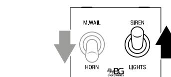
2. While HORN is held down, pull up SIREN. HORN will stop sounding, indicating that you have entered SIREN configuration mode.
