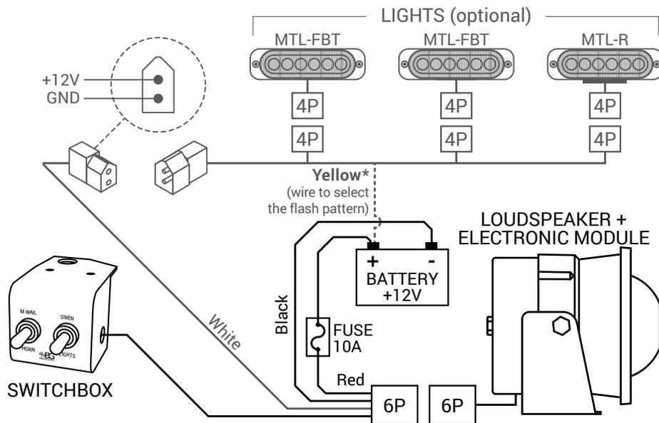
\* The optional lights include 10 flash patterns. To select one, take the yellow wire coming from the harness and connect it momentarily to the power source (12V); the pattern will switch every time the cable makes contact with the source. Once the flash pattern has been selected, make sure to isolate the yellow wire.
