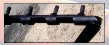
A close up of the side shows the rubber spikes that protrude from the bottom. The rubber spikes are fitted into the receiver and after a few hits require that they be pushed back into the receiver hole.
