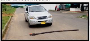
The Spike-Belt is attached to a winder with 80 feet of braided cord. The winder allows the officer to adjust and recover the Spike-Belt from a remote location.
