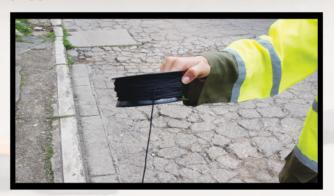
The loop winder style has zero friction for a deployment into far lanes, or across a roadway, officers can move much faster as the cord falls off the edge. Loop winder offers much quicker operation and keeps your eyes off the winder for a better situational awareness.
